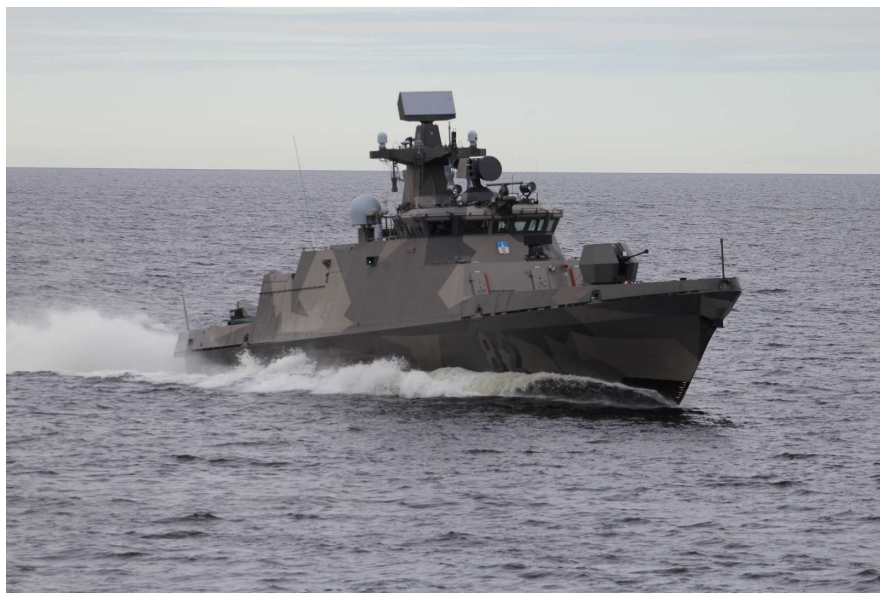
Figure 12: The Hamina-class fast attack craft FNS HANKO is in many ways typical of the escorts available to the navies of the Baltic Sea. The vessel has the ability to counter threats on and below the surface, as well as from the air, but has a limited endurance and magazine depth due to its size, and some key systems are lacking in range. Credit: Robin Häggblom/Risk Intelligence A/S
