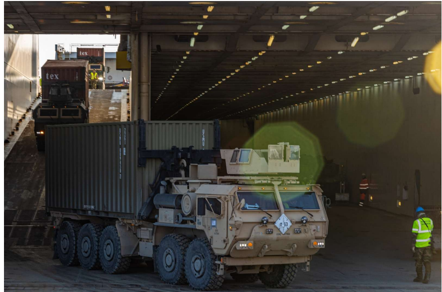
Figure 16: While Ro-Ro vessels in many ways offer the most efficient method of loading and unloading vehicles from a vessel, it is still not a completely straightforward operation, as demonstrated by this USMC LVS manoeuvring between the upper and lower vehicle decks on the Ro-Ro vessel M/V NEW AMSTERDAM while disembarking in Norway. Credit: U.S. Marine Corps photo by Lance Cpl. Christian Salazar
