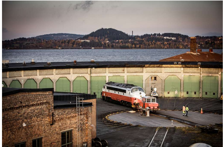
Figure 21: The Östersund locomotive depot houses the workshops of Inlandsbanan AB, and include a planned but not completed drive-through track at one end to better facilitate overhaul of complete train sets including carriages. Note the older Nohab Di3 diesel-electric locomotive, a surplus locomotive doing service on the Inlandsbanan track long after the original user Norges Statsbaner (now Vygruppen AS) has retired the type. Credit: Håkan Wike/Inlandsbanan AB
