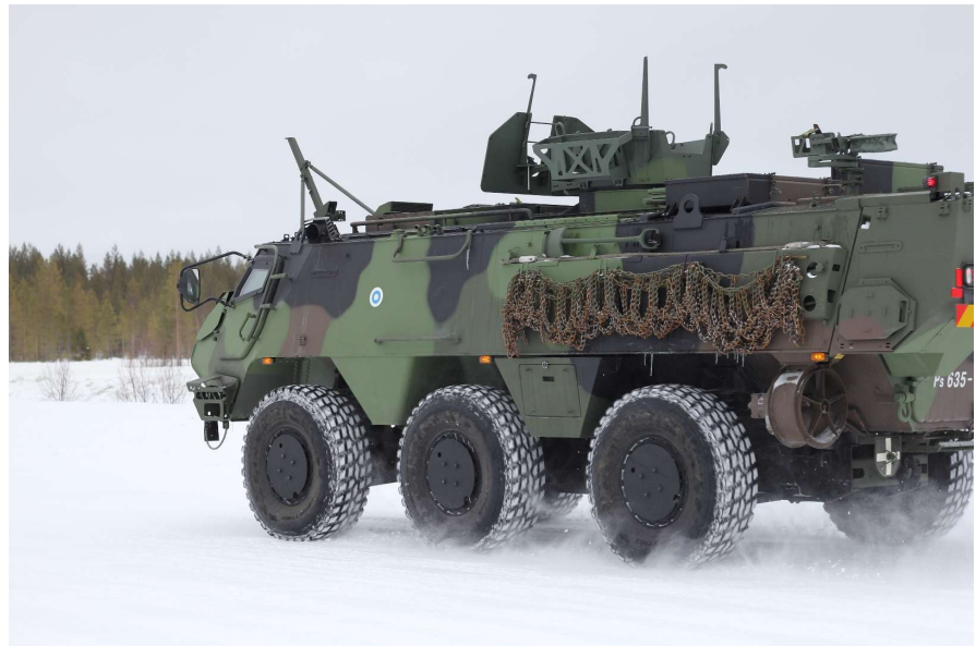
Figure 14: Armoured personnel carriers such as the Patria 6x6 of the CAVS programme are ubiquitous to many military units, including both motorised and mechanised ones. The 6x6 comes in at 15.5 tons empty, and at 7.5 meters long and 2.9 m wide is roughly similar in size to many trucks found on the roads. Credit: Robin Häggblom/Risk Intelligence A/S
