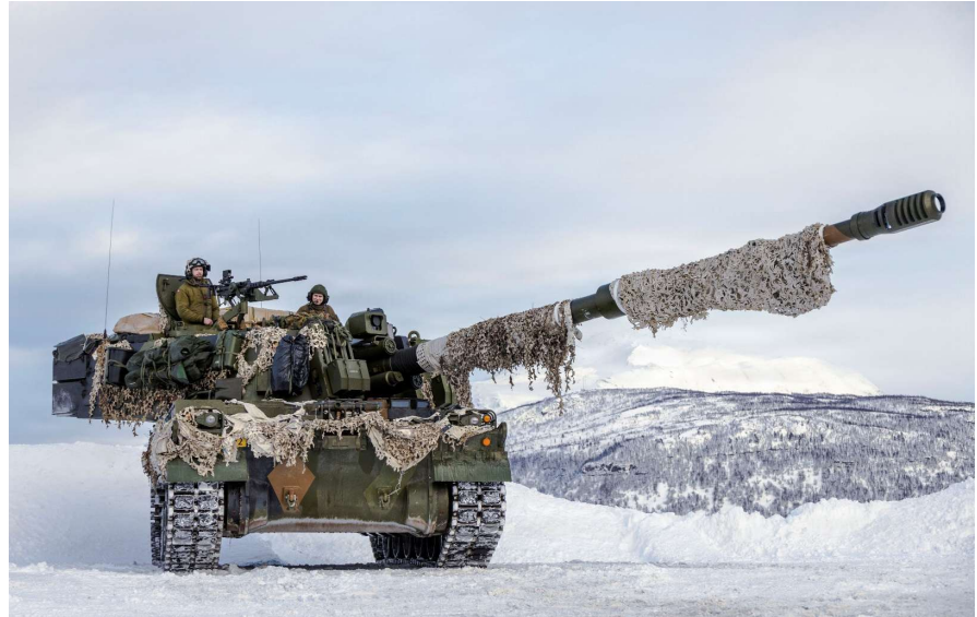
Figure 15: Although not on par with modern main battle tanks, self-propelled artillery such as this Norwegian K9 Thunder 155 mm tracked howitzer with a weight of 47 tons are some of the heaviest vehicles on the modern battlefield. Credit: U.S. Marine Corps photo by Sgt. Addysyn Tobar
