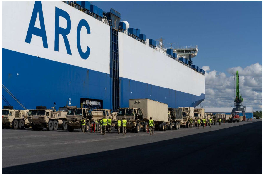
Figure 5: The Ro-Ro MV ARC INTEGRITY is typical of the large car and truck carriers which have capacity measured in thousands of vehicles, in the case of MV ARC INTEGRITY she is able to carry 8,000 cars. Here she is employed during exercise DEFENDER 24, having unloaded part of the heavy vehicles of a US Army Transportation Battalion in a Finnish port. The vehicles are staged on the open quay, before moving out. Credit: U.S. Army photo by Eugen Warkentin
