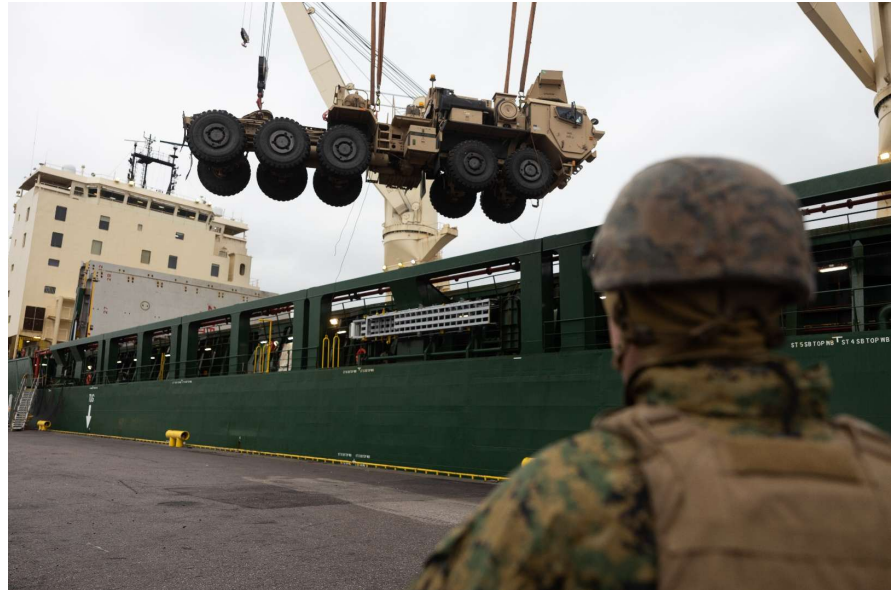
Figure 4: Unloading of a 23-ton curb weight LVSR over the side of the vessel using the ship's own crane. Lo-Lo handling is more often associated with containers and other forms of break bulk, but can be used for vehicles as well. In particular for heavy vehicles or if the port of debarkation lacks a suitable Ro-Ro ramp it can be the preferred option. Credit: U.S. Marine Corps photo by Cpl. Apollo Wilson
