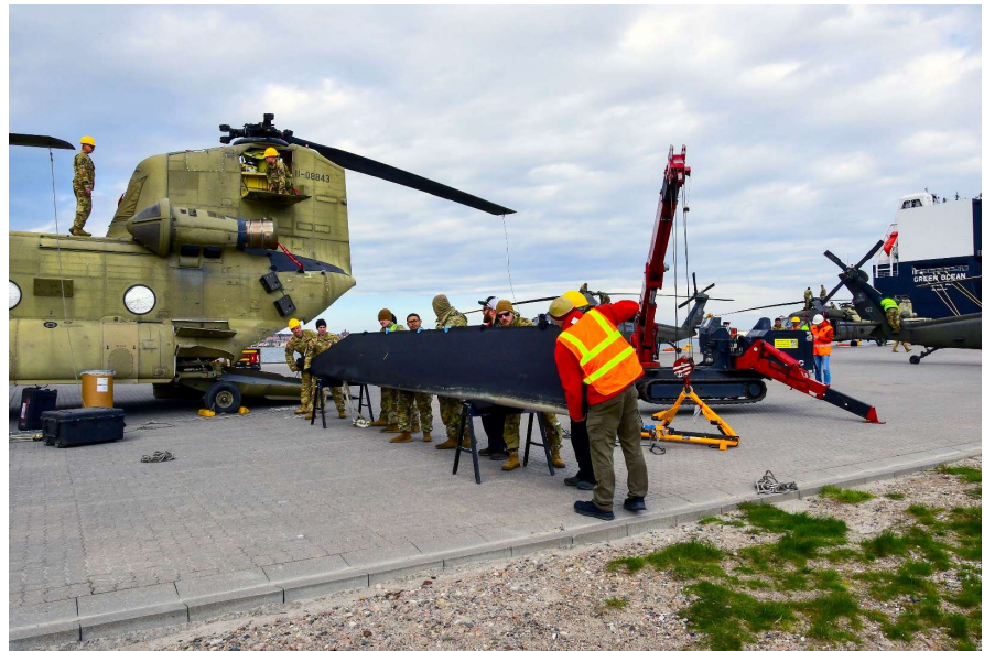
Figure 7: Soldiers and civilian technicians at work attaching the rotor blades on a US Army CH-47F Chinook after it has been unloaded from the Ro-Ro vessel MV GREEN OCEAN in the Danish port of Kalundborg. Due to their limited range, helicopters most often are transported into the theatre as cargo aboard ships or large military transport aircraft, and then require a certain amount of reassembly and overhaul before they are ready for usage. Due to their great mobility once in the theatre of operations, helicopters can use ports of disembarkation further back without this leading to additional delays or undue load on the local transport infrastructure, in contrast to many ground units. Credit: U.S. Army photo by Elena Baladelli
