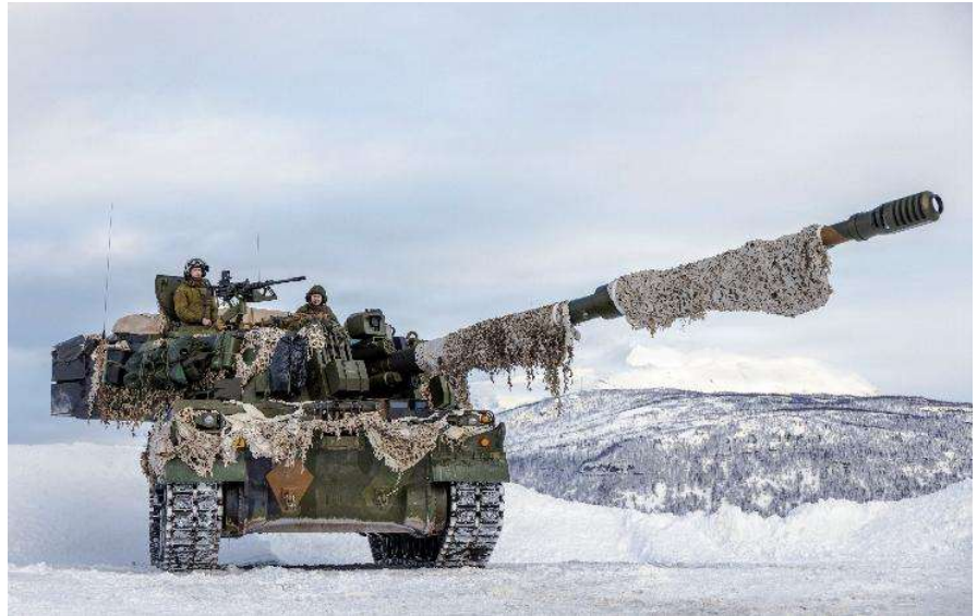
Figure 5: Although not on par with modern main battle tanks, self-propelled artillery such as this Norwegian K9 Thunder 155 mm tracked howitzer with a weight of 47 tons are some of the heaviest vehicles on the modern battlefield. Credit: U.S. Marine Corps photo by Sgt. Addysyn Tobar
